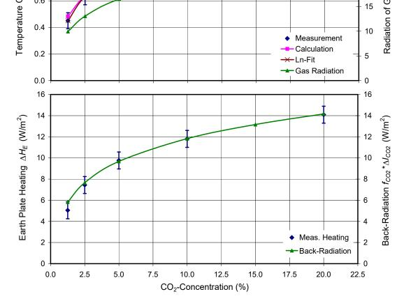
Figure 7: a) Measured temperature change of the earth-plate as a function of the CO<sub>2</sub>-concentration in dry air (Blue Diamonds) and calculation (Magenta Squares). Superimposed is a logarithmic fit (Brown Crosses) and the LBL-RT-calculation of the back-radiation  $\Delta I_{CO2}$ . b) Comparison of measured plate heating  $\Delta H_E$  (Blue Diamonds) and calculated back-radiation collected by the earth plate  $f_{CO2}$ - $\Delta I_{CO2}$  for  $f_{CO2} = 0.59$  (Green).
