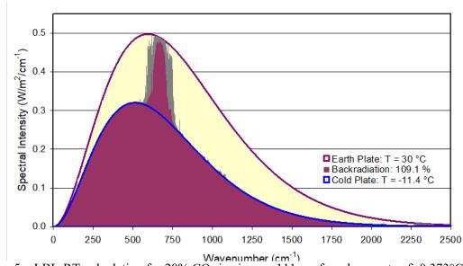
Figure 5: LBL-RT-calculation for 20% CO<sub>2</sub> in air over 111 cm for a lapse rate of -0.373°C/cm: Back-radiation from cold plate and gas (Plum-Gray), radiation only from cold plate (Blue) and spectral intensity of earth-plate (Red-Yellow).
