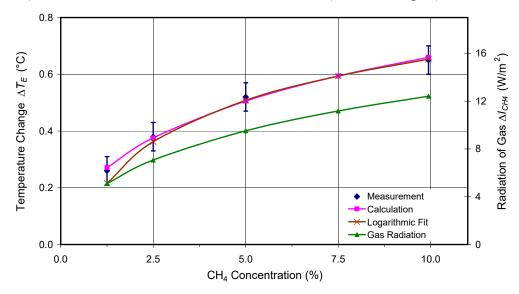
Figure 8: Measured temperature variation of the earth-plate as a function of the CH<sub>4</sub>-concentration in dry air (Blue Diamonds) and calculation (Magenta Squares). Superimposed is a fit assuming a logarithmic function (Brown Crosses) and the LBL-RT-calculation of the back-radiation  $\Delta I_{CH4}$  (Green Triangles).
