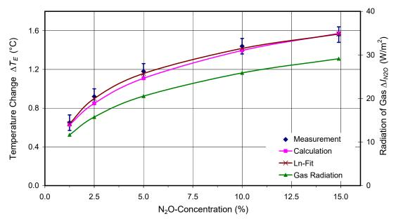
Figure 9: Measured temperature change of the earth-plate as a function of the  $N_2O$ -concentration in dry air (Blue Diamonds) and calculation (Magenta Squares). Superimposed is a fit with a logarithmic function (Brown Crosses) and the LBL-RT-calculation of the back-radiation  $\Delta I_{N2O}$  (Green Triangles).
