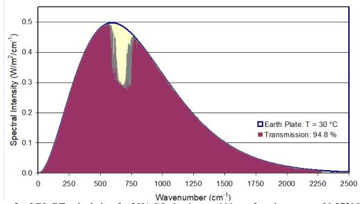
Figure 3: LBL-RT-calculation for 20% CO<sub>2</sub> in air over 111 cm for a lapse rate of 0.373°C/cm. Plotted is the blackbody radiation for 30°C (Blue-Yellow) and the transmitted spectral intensity (Plum-Gray).
