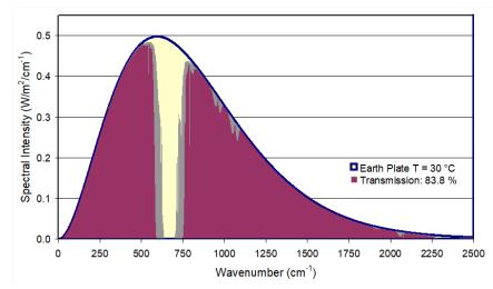
Figure 2: Spectral intensity radiated by the earth-plate at  $T_E$  =30°C (Blue Graph) as a function of wavenumbers. Transmission of initial radiation through 20% CO<sub>2</sub> in dry air at a temperature of 20°C and over a pathlength of 111 cm is shown in Plum color.
