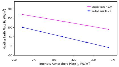
Figure 4: Measured heating of earth-plate for a fixed temperature  $T_E$  of 30°C as a function of the radiated intensity  $I_A$  of the atm-plate (Magenta Diamonds). Also plotted is the expected heating for  $f_A = 1$  (Blue Squares).
