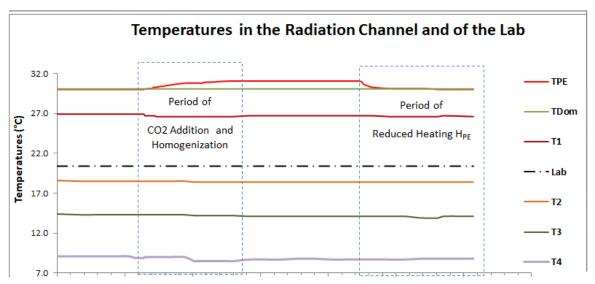
Figure 6: Typical measurement cycle, here for 10% CO<sub>2</sub> in dry air. Plotted are the temperatures of the earth-plate (Red), the dome (Green), the gas temperature at 4 positions  $T_1$  -  $T_4$  (see Fig. 1) and the laboratory temperature (Black).
